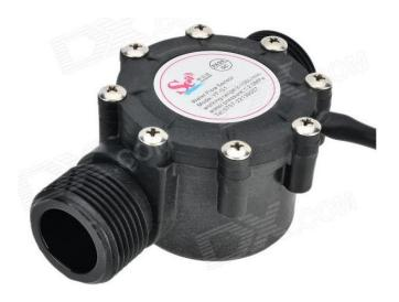
Water flow sensor consists of a plastic valve body, a water rotor, and a hall-effect sensor. When water flows through the rotor, rotor rolls. Its speed changes with different rate of flow. The hall-effect sensor outputs the corresponding pulse signal. This one is suitable to detect flow in water dispenser or coffee machine.
